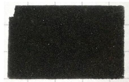
Fig.2: One-layer Ti64-photopolymer composite produced by Digital Light processing
